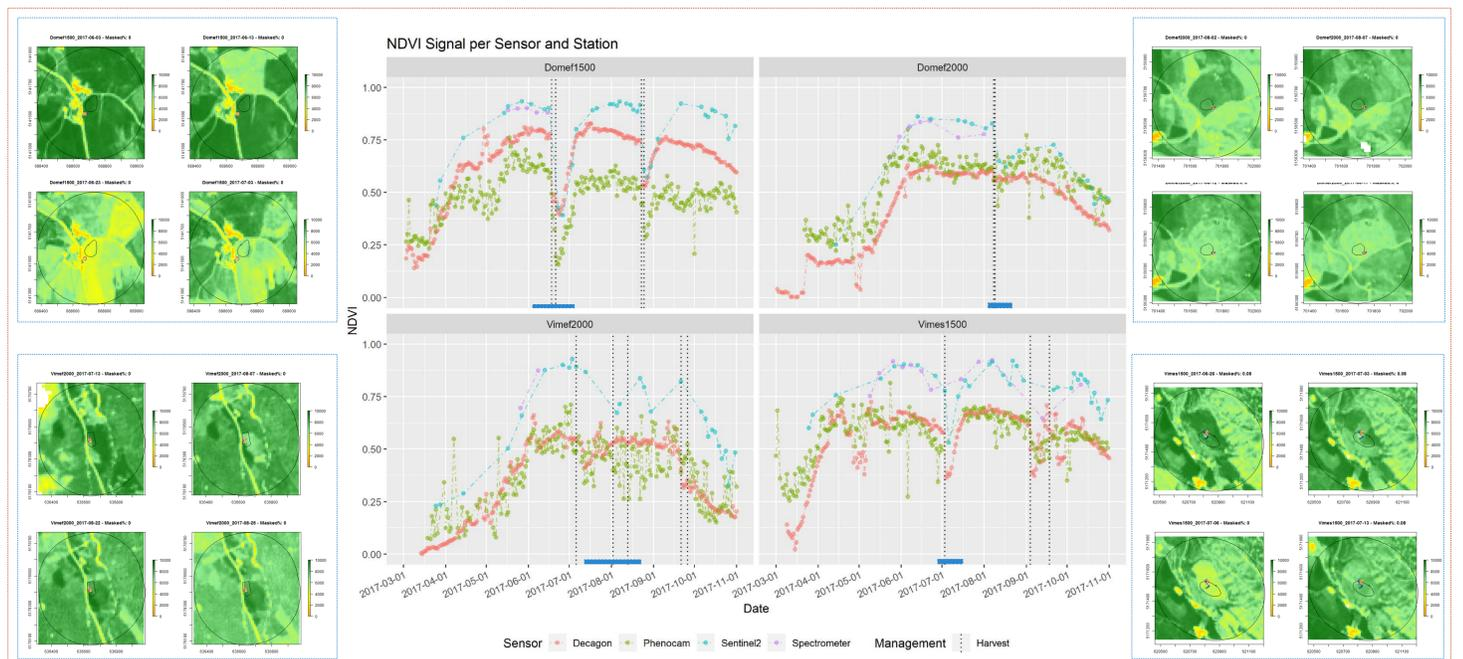
Figure 3: NDVI signatures for each station in 2017 (middle) together with the scaled NDVI derived from Sentinel-2 images during a harvesting event (side)
