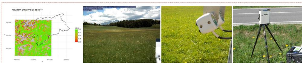
Figure 1: NDVI from Sentinel 2 T32TPS Tile, Phenocam Image, Decagon SRS Sensor and Spectroradiometer
